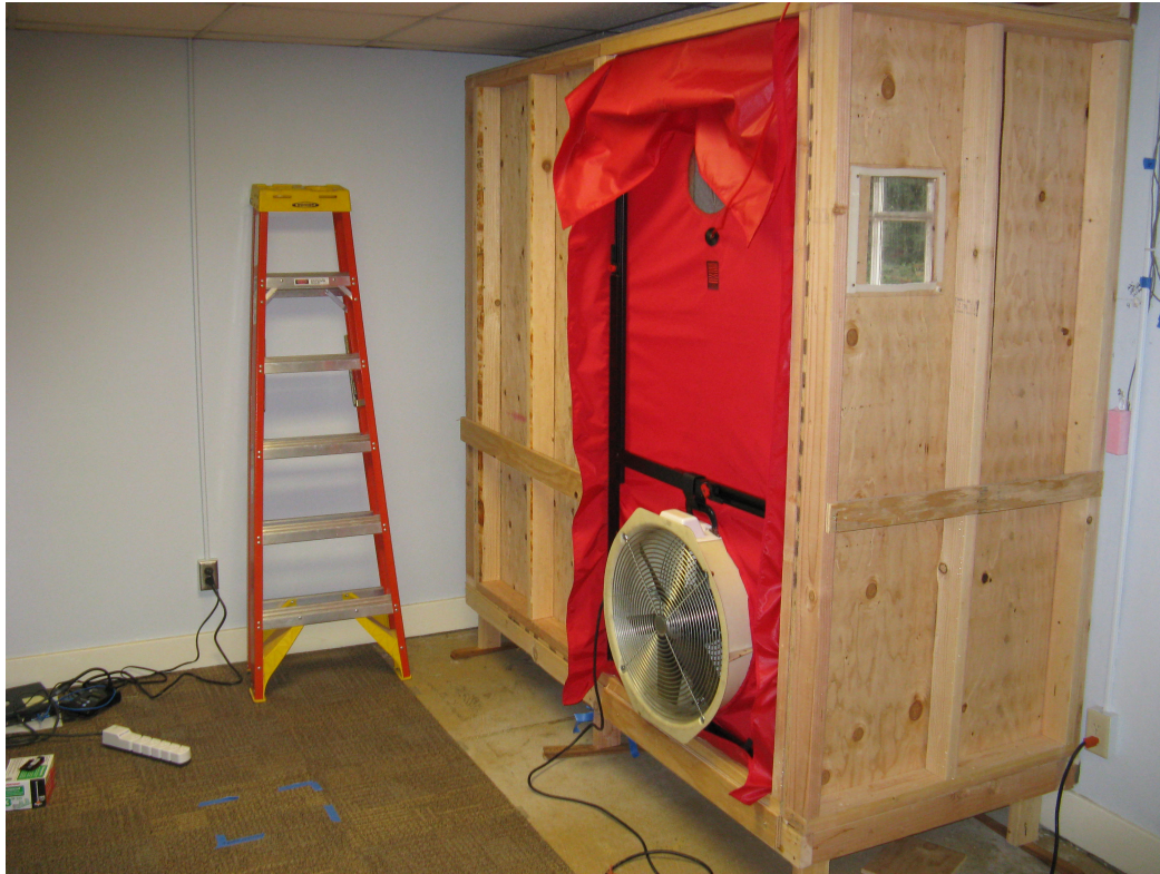
Figure 4, Blower Door Testing in Meter Chamber
